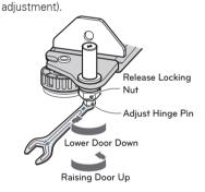
(3) After adjusting door height, firmly tighten the Locking nut ( ) counter-clockwise until secured.
