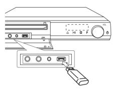
Removing the USB Device from the unit
