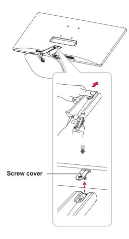
3 Remove the two screws on the back of stand body.
