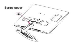
3 Remove the two screws on the back of stand body.
