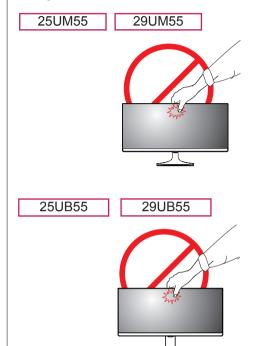
If you use the monitor panel without the stand base, its joystick button may cause the monitor to become unstable and fall, resulting in damage to the monitor or human injury. In addition, this may cause the joystick button to malfunction.
