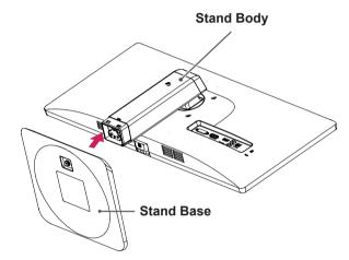
3 Using a coin, turn the screw clockwise to secure the stand base.
