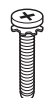
Stativskruvar 2EA, M4 x L20 (Endast 32/39LB58**-ZM) 4EA, M4 x L20 (Endast 32LB57**, 32LB58**-ZA/ZB/ZG/ZJ)
