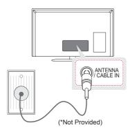
Connect the TV to a wall antenna socket with an RF cable (75  $\Omega).$
