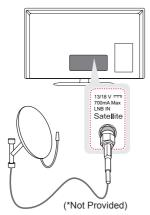
Connect the TV to a satellite dish to a satellite socket with a satellite RF cable (75  $\Omega$ ).
