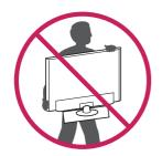
Hold the top and bottom of the TV frame firmly. Make sure not to hold the transparent part, speaker, or speaker grill area.
