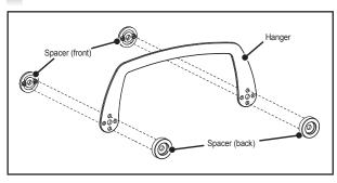
→ Attach the spacers to the hanger in the direction of the dotted lines as shown in the illustration
