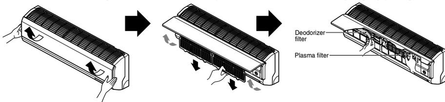
**Type 2:** Pull the front panel from both sides as shown.
