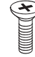
Aluse kruvid 4EA, M4 x L10 (Ainult UB85**-ZD, UB95**-ZB, UC97**) (Vt lk A-4, A-7)
