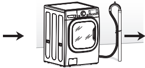
Connecting the drain line
