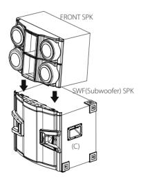
3. FOOT (A) of FRONT SPK is mounted on the top of the guide hole (B) of SWF(Subwoofer) SPK.
