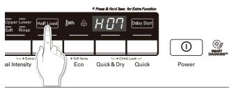
Press the Half Load button, and then set up your intended value. (Scope of setting value : H00~H07)
