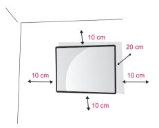
Install the monitor at least 10 cm away from the wall and leave about 20 cm of space at each side of the monitor to ensure sufficient ventilation.
