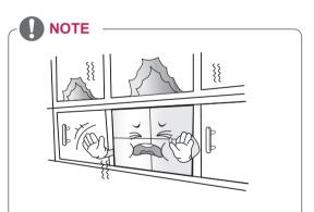
Do not install the product in a place with no ventilation (e.g., on a bookshelf or in a closet) or on a carpet or cushion. If there is no other option but to mount the product on the wall, make sure that sufficient ventilation is provided before installation.
