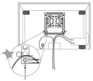
Prevent the power cord and the cables from being pinched between the wall mounting bracket and the wall.
