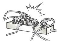
Do not plug too many electrical devices into a single multiple electrical outlet. Otherwise, this may result in fire due to over-heating.
