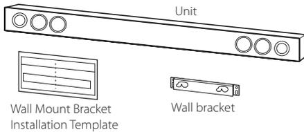
1. Match the TV's BOTTOM EDGE of Wall Mount Bracket Installation Template with the bottom of TV and attach to the position.
