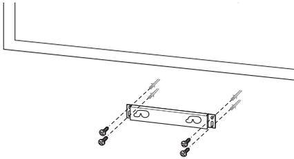
5. Hang the main unit onto the bracket as shown below.
