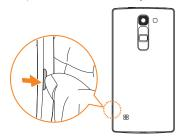
2 Slide the SIM card into the lower slot for the SIM card as shown in the figure. Make sure the gold contact area on the card is facing downward.
