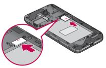
3 Insert the battery into place by aligning the gold contacts on the phone and the battery 1 and press the battery down until it clicks into place 2.
