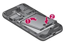
4 Align the back cover over the battery compartment 1 and press it down until it clicks into place 2.
