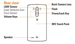
**LDAF Sensor (Laser Detection AutoFocus Sensor):** This sensor measures the distance to the subject using laser technology and allows for improved focusing speed and object detection in low-light situations.
