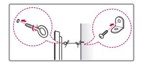
1 Insert and tighten the eye-bolts, or TV brackets and bolts on the back of the TV.
