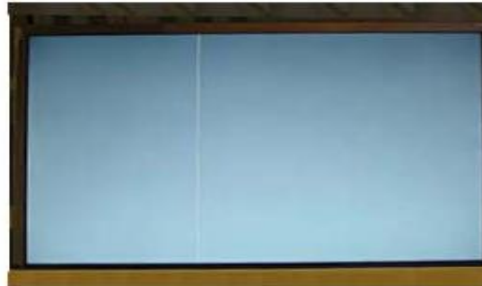
Vertical Line Source TAB IC Defect
