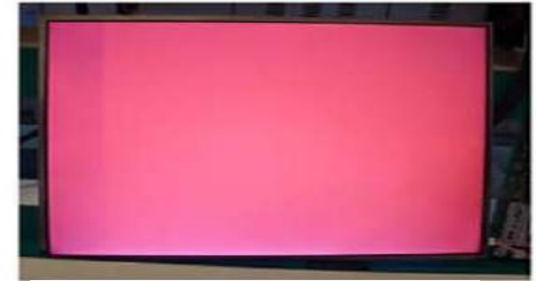
Vertical Block Source TAB IC Defect
