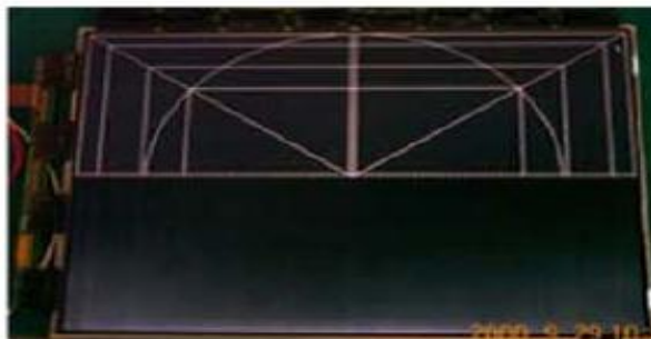
Horizontal Block Gate TAB IC Defect
