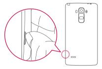
2 Slide the SIM card into the lower slot for the SIM card as shown in the figure. Make sure the gold contact area on the card is facing downward.
