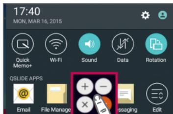
Open the Notifications Panel and tap the desired app from the **QSLIDE APPS** section.
