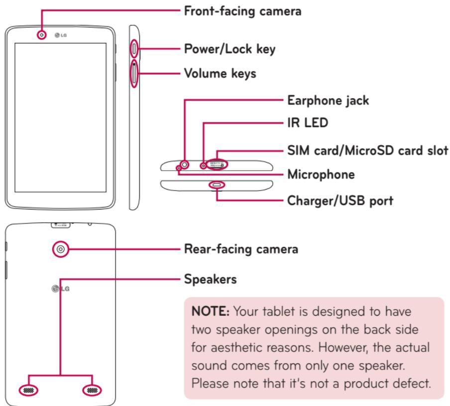
**NOTE:** Your tablet is designed to have two speaker openings on the back side for aesthetic reasons. However, the actual sound comes from only one speaker. Please note that it's not a product defect.
