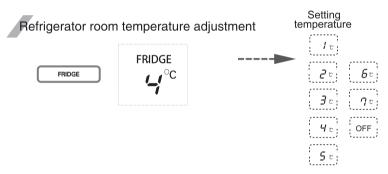
% Whenever pressing button, setting is repeated in the order of  $(4^{\circ}\text{C} \rightarrow 5^{\circ}\text{C} \rightarrow 6^{\circ}\text{C} \rightarrow 7^{\circ}\text{C} \rightarrow 0\text{FF} \rightarrow 1^{\circ}\text{C} \cdots \rightarrow 4^{\circ}\text{C})$ .
