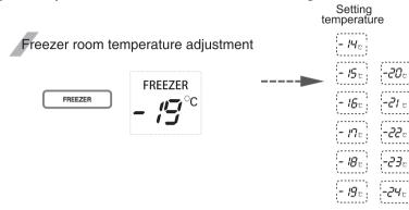
Whenever pressing button, setting is repeated in the order of  $(-19^{\circ}\text{C} \rightarrow -20^{\circ}\text{C} \cdots \rightarrow -24^{\circ}\text{C} \rightarrow -14^{\circ}\text{C} \cdots \rightarrow -19^{\circ}\text{C})$ .
