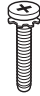
Stand Screws 2EA, M4 x L20 (Only 32/39LB65**-ZE/ZN) 4EA, M4 x L20 (Only 32LB65**-ZA/ZK) (See p. A-3, A-4, A-5)
