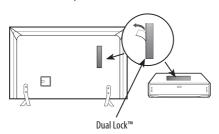
2 Attach the set-top box to the TV by pressing the Velcro strips together.
