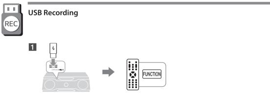
Connect a USB device and select the function (CD, AUX, PORTABLE, Tuner) to record.
