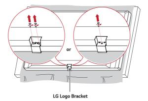
2 After removing the screw, remove the LG Logo Bracket. Attach the LG Logo Bracket with the screws, aligning it with the hole on the right side.
