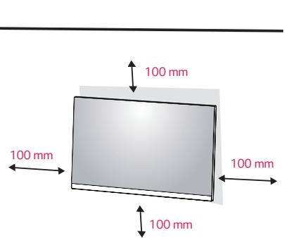
To install the monitor to a wall, attach a wall mounting bracket (optional) to the back of the monitor. Make sure that the wall mounting bracket is securely fixed to the monitor and to the wall.
