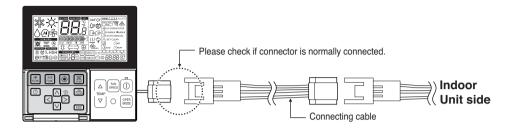
Please use extension cable if the distance between wired remote controller and indoor unit is more than 10m.
