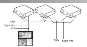
When controlling multiple indoor units with event communication function with one remote controller, you must change the master/slave setting from the indoor unit.
