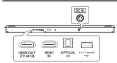
HDMI OUT (TV ARC) ····· Connect to a TV. ····Connect to device with HDMI OUT. OPTICAL IN --······Connect to an optical device. ·····Connect to a USB device. · · Connect to the AC adapter.
