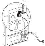
Connect the additionally provided water supply hose of Main Washer to the cold water supply hose connector and cold water tap.
