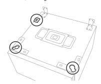
**2** Securely attach the two washer at the corners using screws.
