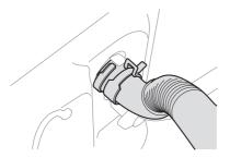
Adjust the band clamp with pliers to keep the hose securely in place and prevent leaking.
