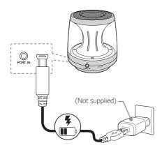
If the battery is fully charged in charging mode, **EED** (RED) is turned off.
