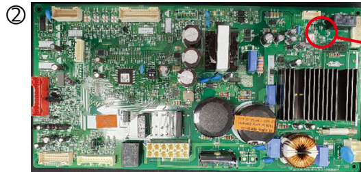
2. Check the number of LED blinks (Refer to the next page for resolution by number of LED blinks)
