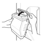
3 Remove the cover while the handle of the water tank is lifted.
