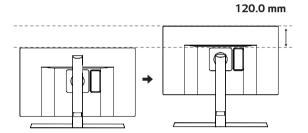
• Do not put your fingers or hand between the screen and the base (chassis) when adjusting the screen's height.
