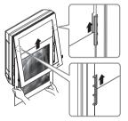
9. Push both links of lower part of panel inside and fix it. Then turn on.
