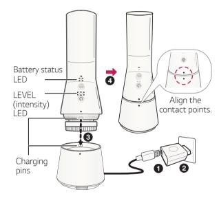
(!) When charging, place the device on the contact point of the charging stand. (Ensure that the contact point of the device and the charging cradle match). When correctly charging, the UV light on the bottom of the charging cradle will be lit.
