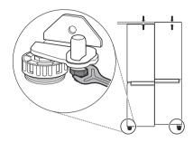
Open the door and use the spanner ① to loosen the keeper nut by turning it to the left.
