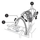
3 Rotate the hinge lever S counterclockwise. Lift the top hinge S free of the hinge lever latch **7**.
