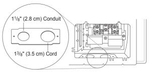
Remove the conduit connection plate
