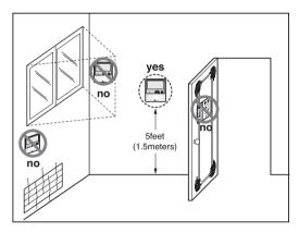
Fig.1 Typical locations for remote controller
