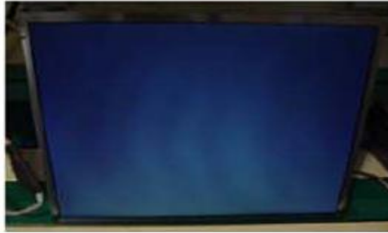
Panel Mura, Light leakage
