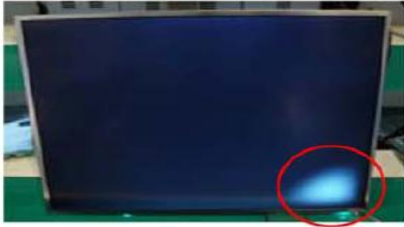
Panel Mura, Light leakage
