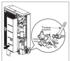
₩ When tighten the pipe, hold the hexagonal body.
