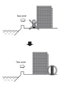
In case, to install the outdoor unit on the seaside, set up a windbreak not to be exposed to the sea wind.
