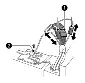
3 Rotate the hinge lever **5** counterclockwise. Lift the top hinge 4 free of the hinge lever latch 3.
