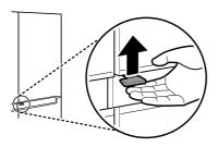
Lift the vegetable drawer up and remove it by pulling it out.
