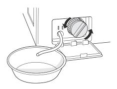
Clean the pump filter and opening.
