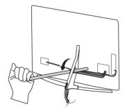
• Do not use a sharp object when you detached the cable cover. This could damage the cable or the cabinet. It may also cause personal harm. (Depending on model)
