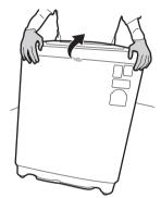
3 Insert the anti-rat cover to the assembling hole at the bottom of the appliance.
