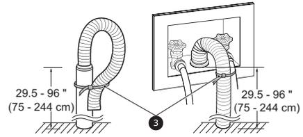
**Using a Laundry Tub to Drain**
