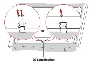
2 After removing the screw, remove the LG Logo Bracket. Attach the LG Logo Bracket with the screws, aligning it with the hole on the right side.
