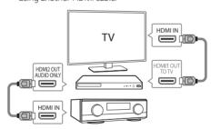
3 Set the input selector to HDMI on the TV and amplifier.
