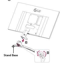
3 As shown in the illustration, pull Screw Cover out to separate it from the set.
