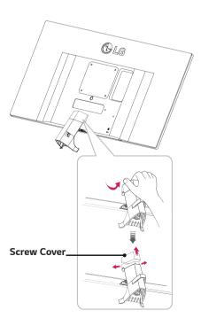
4 Remove the two screws on the back of stand body. As shown in the illustration, disconnect the **stand body** from the **stand hinge**.
